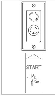
A panic button is integrated in the system. The door that was last used is opened again and the user can leave the system. The information about which door was last opened is stored in the control system as long as the mains voltage is applied.
