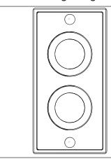
The signal lights indicate the release status for the respective direction of passage. When the signal light is red, the system is blocked for the corresponding direction of passage, and when the signal light is green, the system is released.
