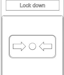
To prevent someone from being locked in the system and to maintain the security of the building, there is a high priority input contact. With this function, one door is closed first before the opposite door is opened.
